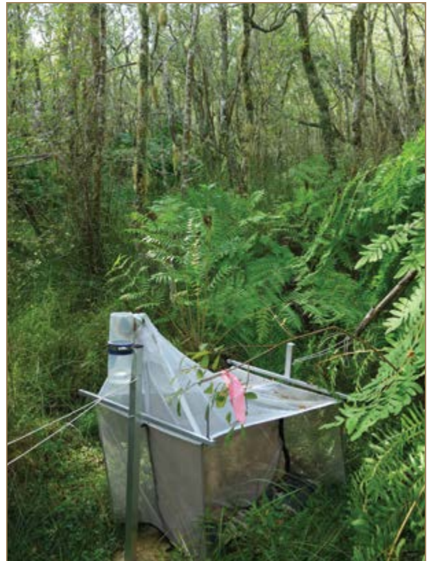
A tent trap for collecting flying insects in Whangamarino. Photo: Danny Thornburrow
