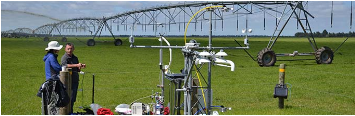
Measurement setup to determine greenhouse gas budgets of irrigated pasture. image - John Hunt
