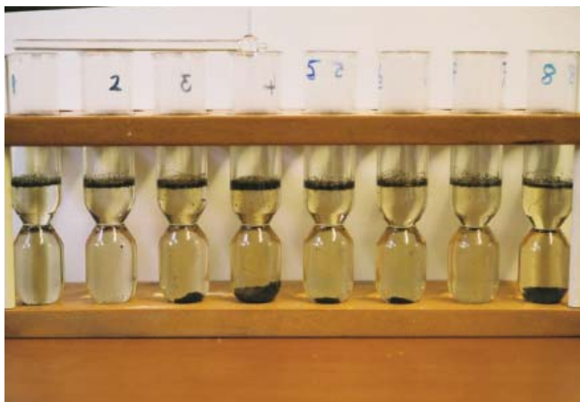
Figure 2: Method to separate different soil fractions
