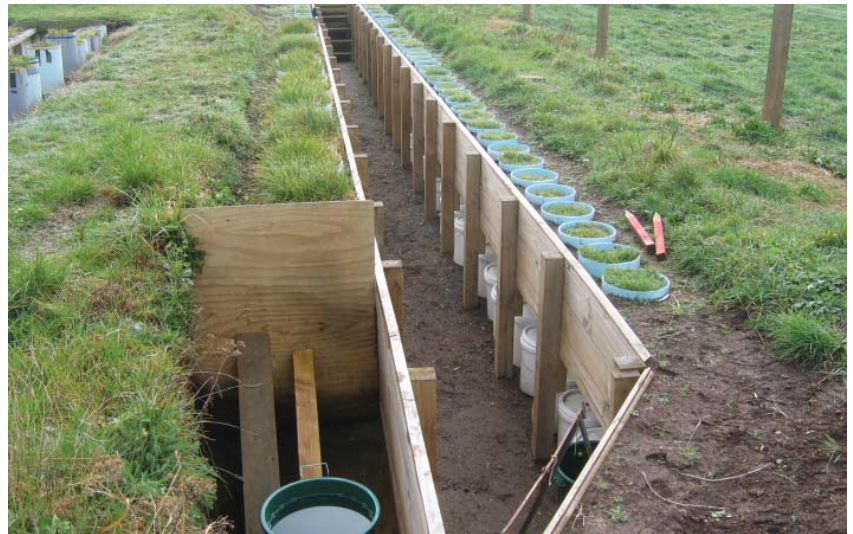
Figure 1: Lysimeters established to investigate nitrogen storage and leaching processes
