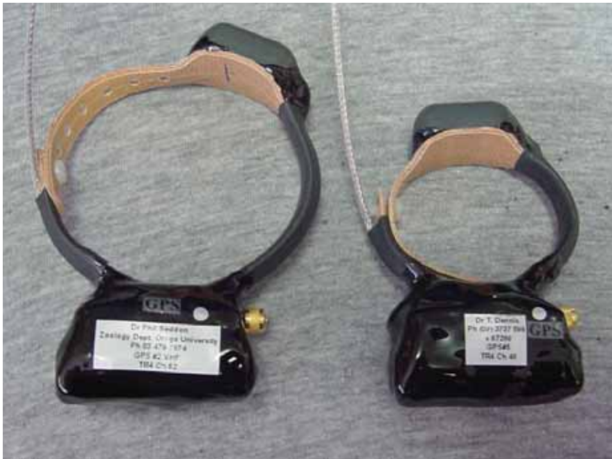
Sirtrack GPS collars for a cat (left) and possum (right).
