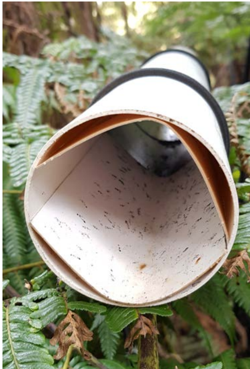
Two inked tracking cards (with adult MGW prints present) are rolled around the inside of the tunnel.
