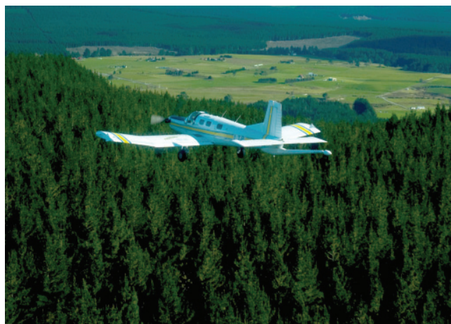
FIGURE 46 Airborne geophysical survey of the Taupo Volcanic Zone in 2005. The magnetometer sensor is mounted in a ‘stinger’ at the rear of the aeroplane. Photo: Glass Earth Gold Ltd.
