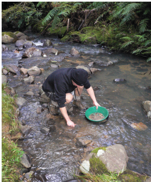
FIGURE 45 Collecting a stream sediment sample for geochemical analysis. Photo: Tony Christie.
