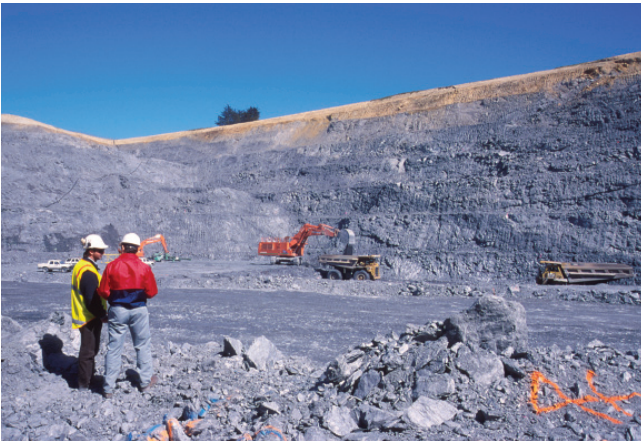
FIGURE 24 Macraes mine, Frasers open pit. The Hyde–Macraes Shear Zone is exposed as a dark grey carbonaceous crush zone dipping to the right on the far wall (above the digger and truck) of Frasers open pit. Photo: Tony Christie.
