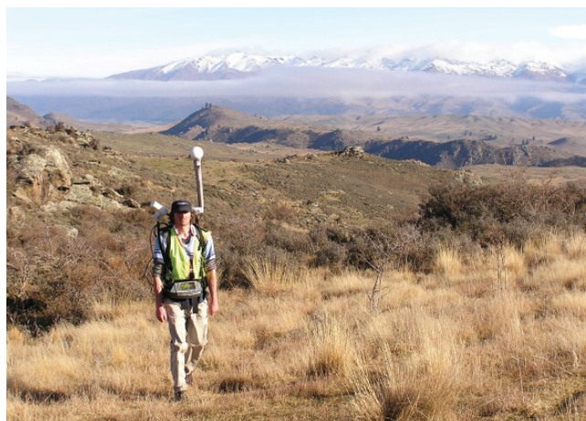
FIGURE 47 Ground magnetic survey, Central Otago. Photo: Glass Earth Gold Ltd.
