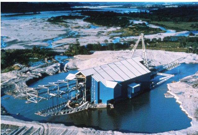
FIGURE 29 A bucket-ladder gold dredge that has worked intermittently in the Grey River since 1992.
